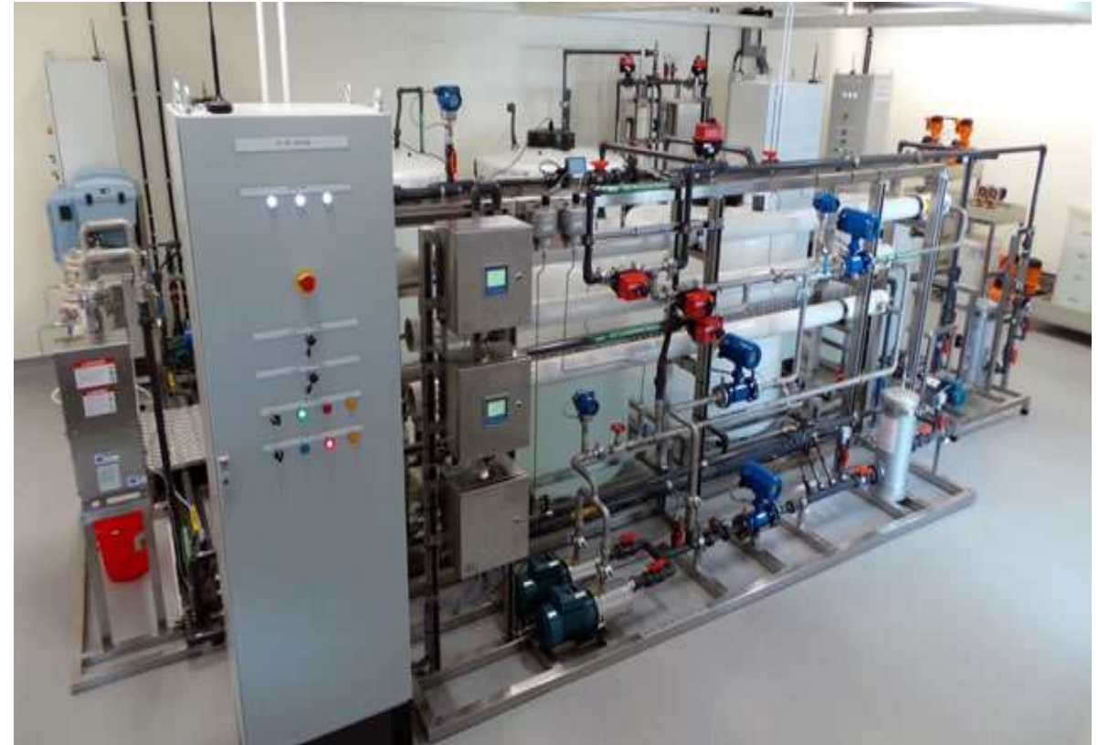
The Secure Water Treatment (SWaT) testbed at the Singapore University of Technology and Design
